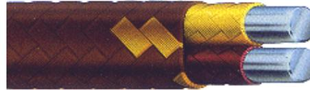
A Thermocouple is a temperature measuring device consisting of two conductors of dissimilar metals or alloys that are connected only at the ends. When the ends are at different temperatures a small voltage is produced in the wire that can be related directly to the temperature difference between the ends. If the temperature at one end is known, the temperature at the other end can be determined.
