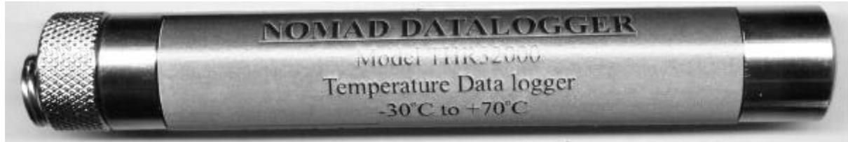
The T-HR is a small Single High Resolution (12 bit) Temperature Datalogger with an internal probe. The Datalogger is housed in a 19mm ( $\frac{3}{4}$ " ) 304 stainless steel tubular case.
